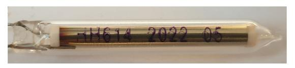
Mhen using the counting tube, ensure that the surface is clean; no impact or mechanical damage; no contact with strong alkalis or acids
